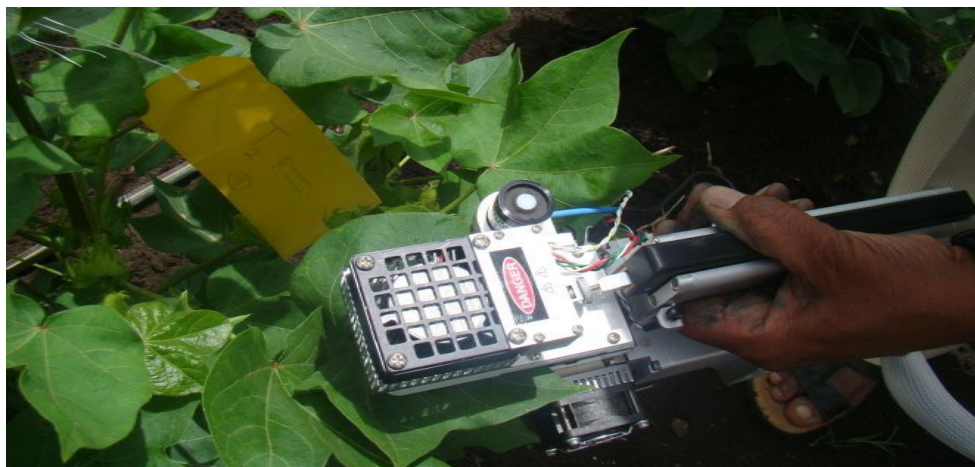
Recording Photosynthesis of cotton with Infra Red Gas Analyser
